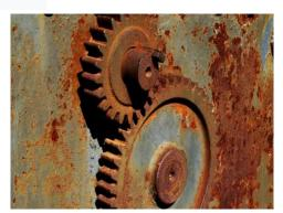
hydrated iron(III) oxides  $Fe_2O_3 \cdot nH_2O$  and iron(III) oxidehydroxide (FeO(OH), Fe(OH)<sub>3</sub>).
